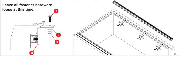
Position assembled side rails from the closed tailgate: With the truck's tailgate closed, position the end of each rail approximately 1/2" away from the rear corner of the truck bed. This positioning helps ensure proper alignment of the rail system and allows for clearance when opening and closing the tailgate.
