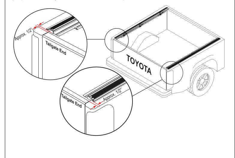
Adjusting the cross car spacing of side rails (A) and (B) at the tailgate end of the truck bed: At this point, the side rails should already be spaced correctly fore and aft (lengthwise), focusing now on the side-to-side spacing at the tailgate end.
