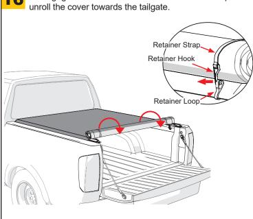
Place the rear header into the header stops which are located on both side rails. Rotate the rear header downwards until you feel the cover latch in place. A clicking sound will indicate a correctly installed cover.
