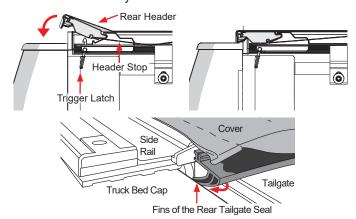
**NOTE:** When you close the tailgate, it pushes the fins toward the inside of the bed with the rest of the seal partially on top of the tailgate.
