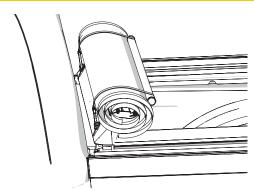
Roll up the cover. Do not disengage the hook and loop fasteners before rolling the cover. Always secure the cover at the front with both retainer straps.
