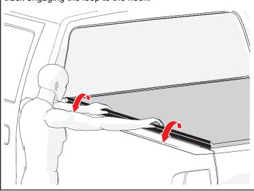
hand to firmly push the loop strip into the hook track. Do this to both driver and passenger sides. You are ready to drive with the cover (C) in the closed position.
