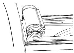
Roll up the cover (C). Do not disengage the hook and loop fasteners before rolling the cover. Always secure the cover at the front with both retainer straps.
