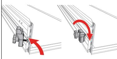
Position the buckle ends (I) with the open side facing the bed cover panel. Use a screwdriver to install the two buckles into the pre-drilled holes on the front header panel with the provided screws (J). **DO NOT use a screw gun, securely tighten by hand only.**
