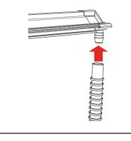
Before placing the cover (A) onto the vehicle, slide two front cover retainer clamps (G) into the track on the underside of the cover (A) near the cab. Confirm the cover retainer clamps fit properly into the cover rail for optimum fit. Repeat on the opposite side of the cover.
