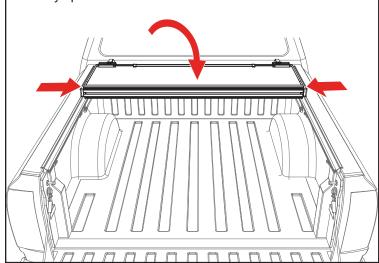
Confirm the retainer clamps (G) are positioned around the side rails (B & C) correctly as shown below. Tighten the retainer clamps by turning them clockwise until the lock washer is secure.
