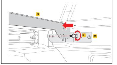
Install the adaptor rail driver side (D) by lining up the studs with the holes in the rear bracket using two M6 flange mounting bolts (K) and two 1/4-20 nuts (L). Repeat on the opposite side using the passenger side adaptor rail (E). Now tighten, using a 7/16" socket in front and rear on both sides.
