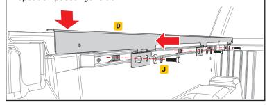
When you get the adaptor rail driver side (D) and the T-nut kits (J) lined up you can now tighten the bolts while you are applying downward pressure to the rail. A second set of hands may help. Repeat on the opposite side using the adaptor rail passenger side (E).
