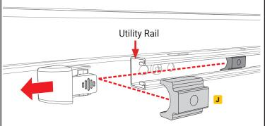
Installing Adaptor Rail: Install adaptor rail driver side (D) with the bolt, washer and lock washer that is attached to the T-nut kit (J) and push the rail all the way toward the cab and the bulkhead. Adjust the t-nuts so they are lined up with the holes in the adaptor rail.
