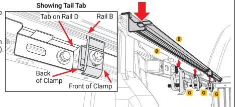
**NOTE:** If the rails are leaning down, have one person stand on the outside of the bed and slightly roll the rails upward while another person slowly snugs the clamps up. If the clamps are tightened too quickly or overtightened, it will cause the rails to lean down.
