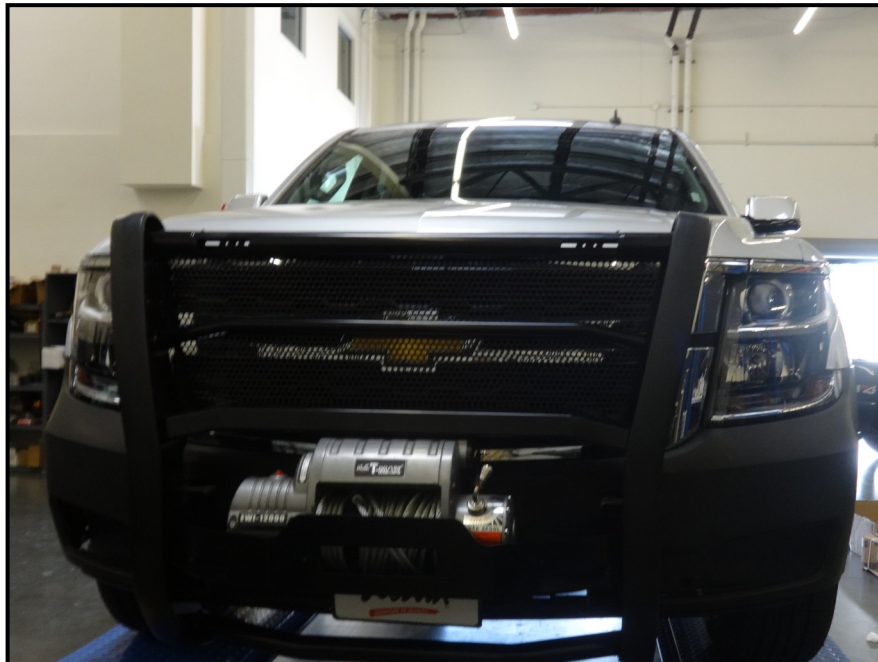
PUSH BAR WITH WINCH TRAY INSTALLATION COMPLETE
