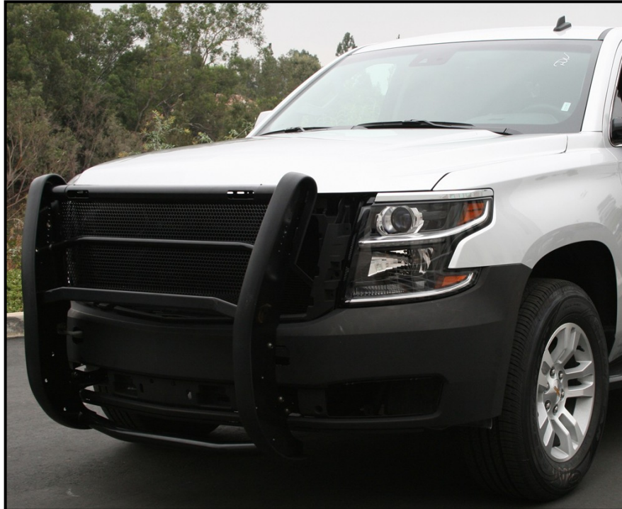
PUSH BAR INSTALLATION COMPLETE
