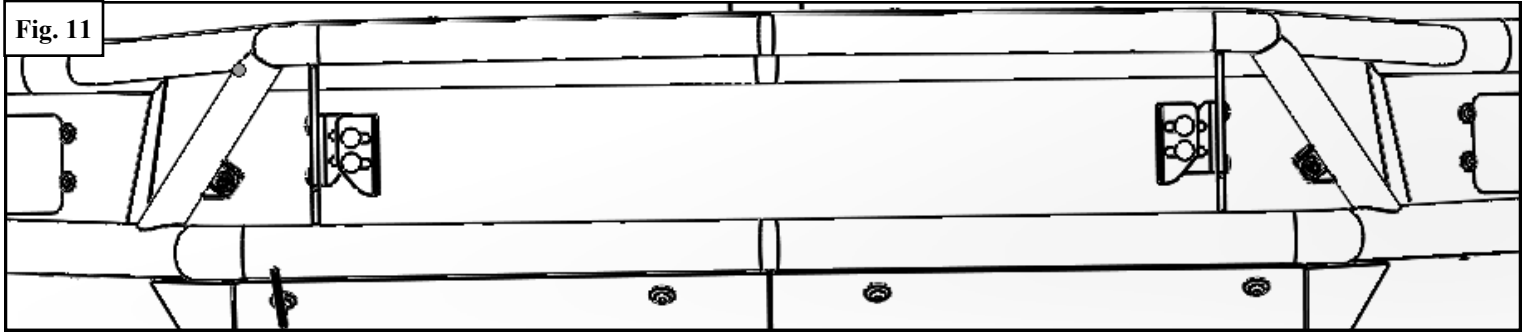
Figure 11 is an example showing the LED brackets adjusted in for the shortest light bar configuration.
