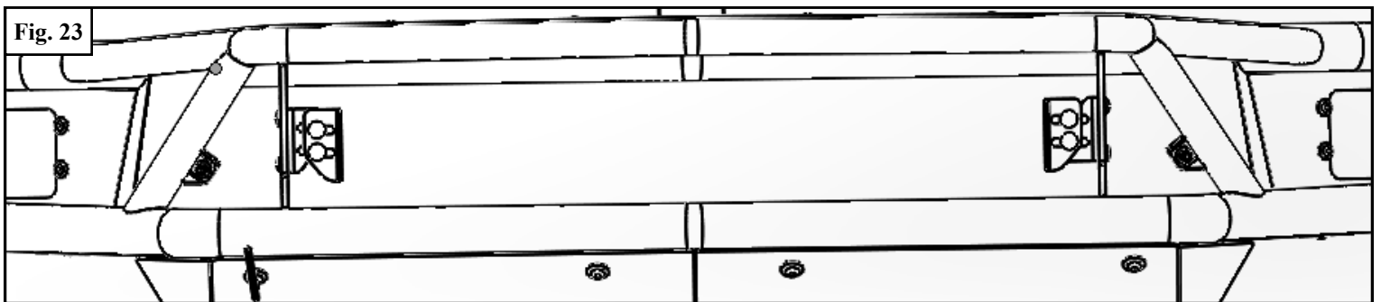
Figure 23 is an example showing the LED brackets adjusted in for the shortest light bar configuration.
